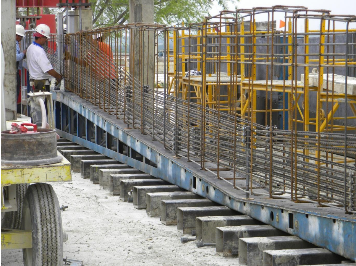
Fig. 11 Strand Layout for Exterior Floor Beam
