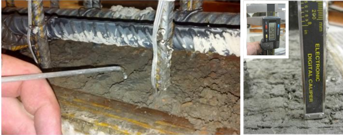
Fig. 4 Interface roughening procedure (left) and measurement (right)
