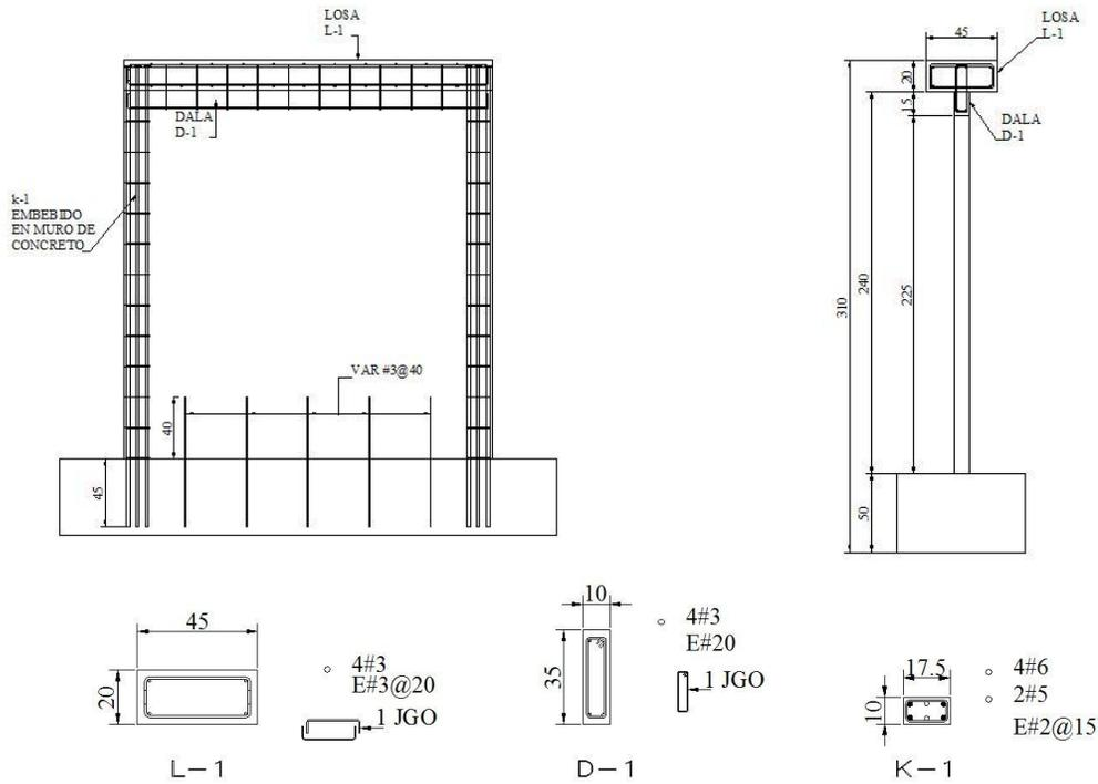
**Figure 9 Wall Reinforcement**
