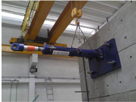
**Figure 3 hydraulic actuator ( 50 t)**
