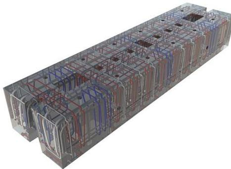
**Figura 10 Foundation Reinforcement**
