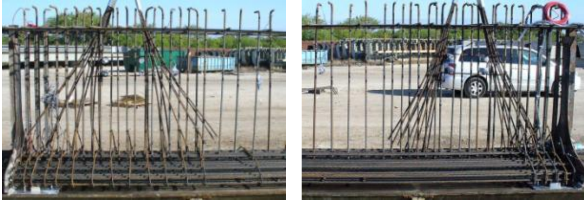
Figure 8 - Reinforcement for specimen DC (left) and specimen DM (right). Specimen DM had more confinement reinforcement (by cross sectional area) near the end. Specimen DC had more confinement reinforcement overall.
