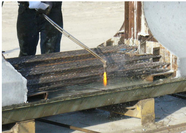
Figure 7 – Prestress transfer by flame cutting strands. Specimens were built simultaneously on the same prestressing line.
