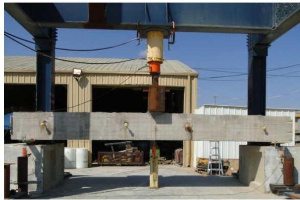
(c) Flexure-shear test setup
