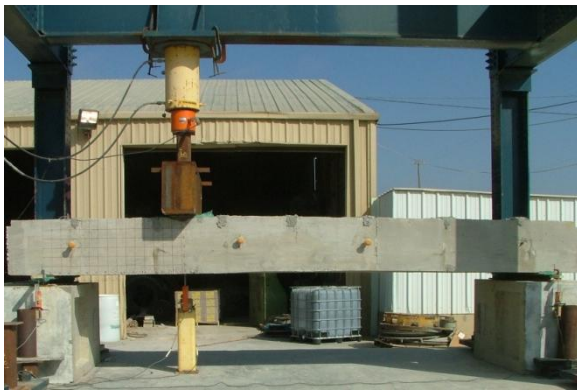
(b) Web-shear test setup
