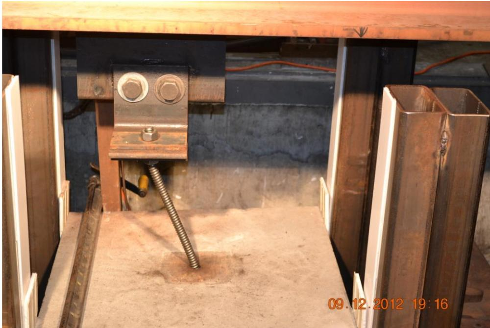
**Figure 4. Fracture of 3/4-inch Coil Rod, 16-inch long Specimen**
