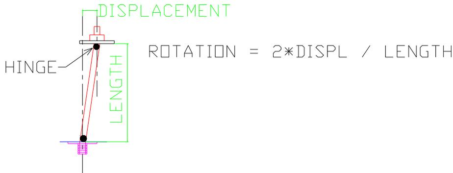
**Figure 7. Proposed Rigid Bar Concentrated Inelastic Hinge (RBCIH) Model for Coil Rod Behavior.**
