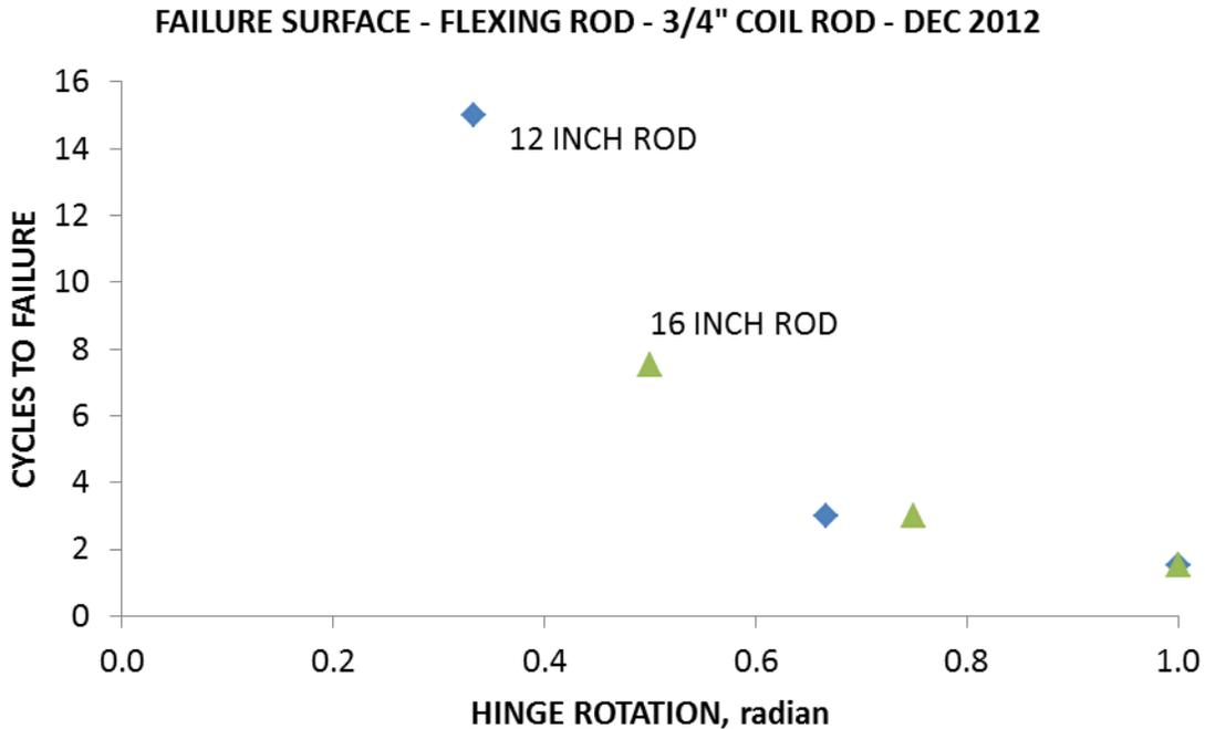
**Figure 8. Prediction of Cycles of Failure based on Peak Hinge Rotation**
