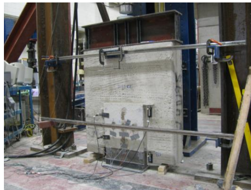
Fig. 12: Push-off test setup
