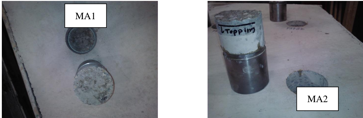
(a) Interface failure
