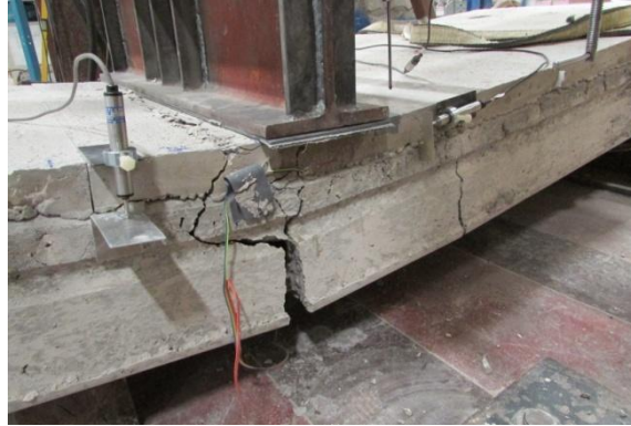
Fig. 23: Slab at failure
