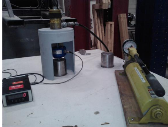
Fig. 6: Pull-off test setup
