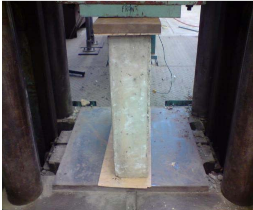
Fig. 3 Post-Fire Concrete Panel Test under Compression
