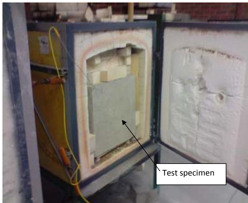
Fig. 2 Test Panel Set for Exposure to Fire
