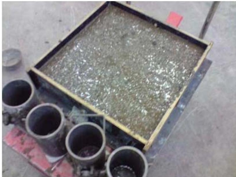
Fig. 1 Casting of a Geopolymer Concrete Test Specimen
