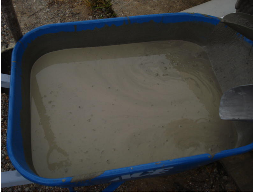
Fig. 4 Segregation Observed in Trial Batch
