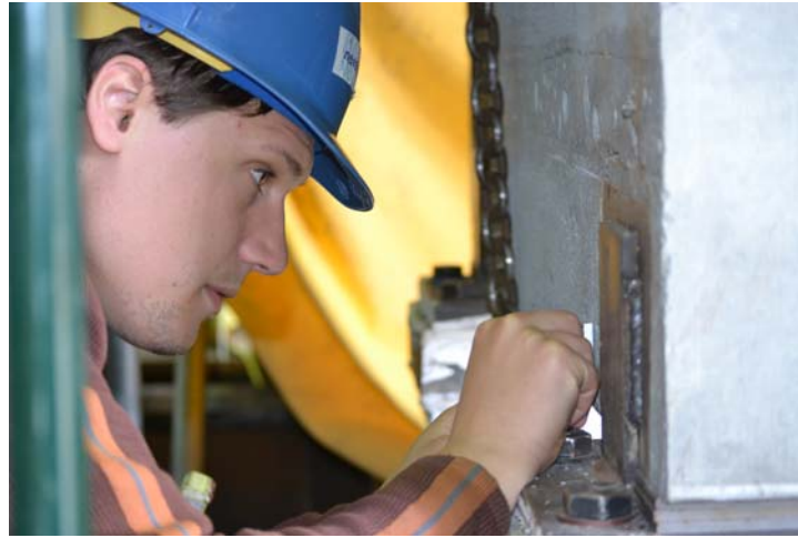
Figure 11. Installation of Wire Transducers for Measurement of Global Movement of Panel
