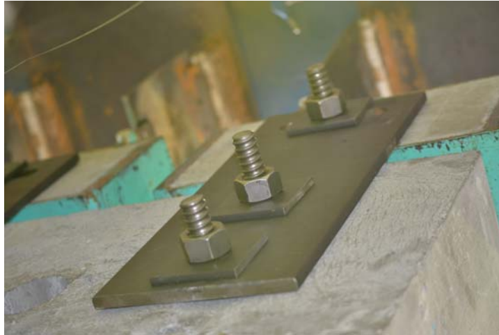
Figure 7. Welded Plate Connection at Base of Column Cover (welded vertical plate represents connection of cladding panel to foundation, for testing, the vertical plate is welded to a flat horizontal plate that is bolted to the load cell to measure forces and bending moments)
