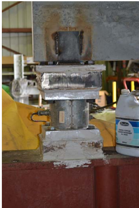
Figure 7. Welded Plate Connection at Base of Column Cover (welded vertical plate represents connection of cladding panel to foundation, for testing, the vertical plate is welded to a flat horizontal plate that is bolted to the load cell to measure forces and bending moments)
