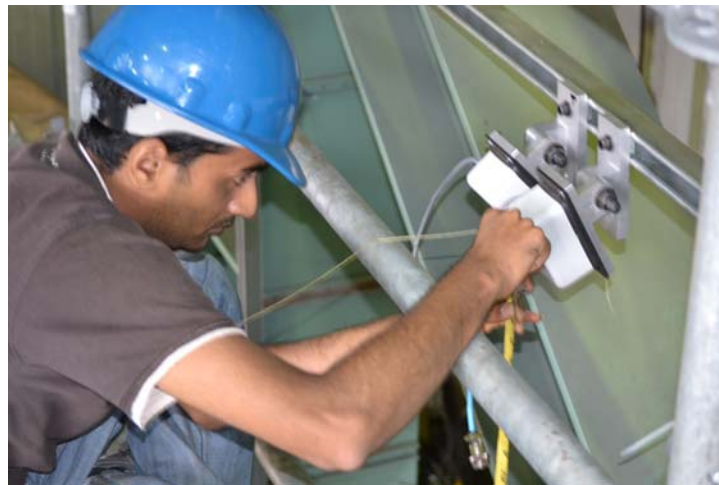
Figure 11. Installation of Wire Transducers for Measurement of Global Movement of Panel
