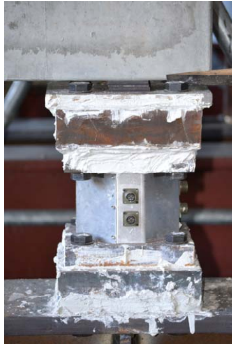
Figure 9. Five-Directional Load Cell at Base of Panel
