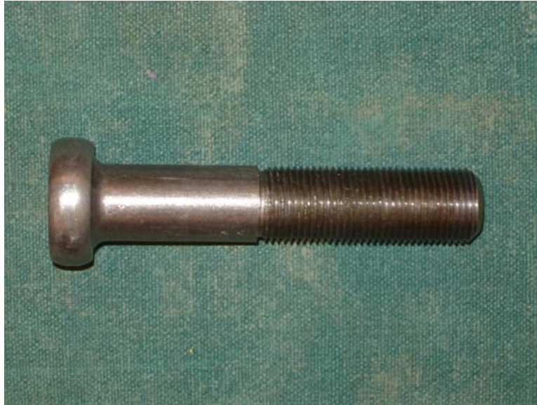
Fig. 1 Headed Stud after Fabrication
