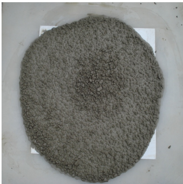
Figure 5. Slump Flow of Final Expanded Shale Mixture
