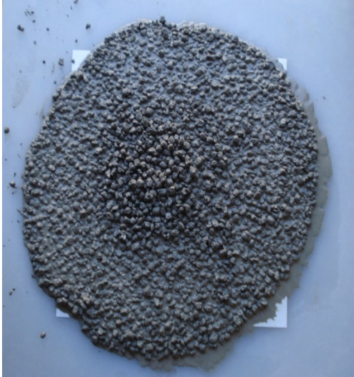
Figure 4. Slump Flow of Final Expanded Clay Mixture
