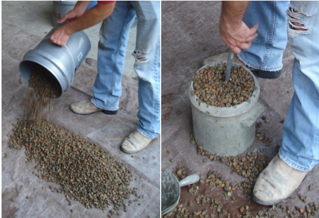
Figure 1. Aggregate Preparation and Unit Weight
