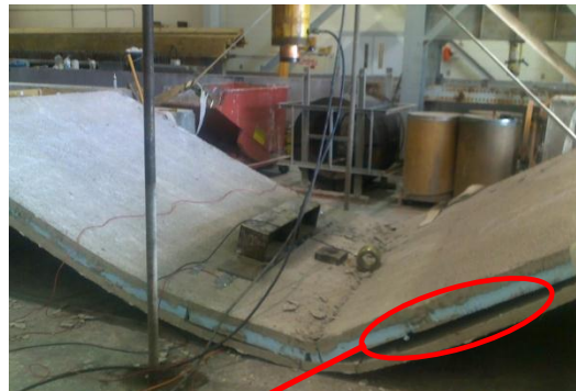
Figure 8: Testing and failure mode of panel A
