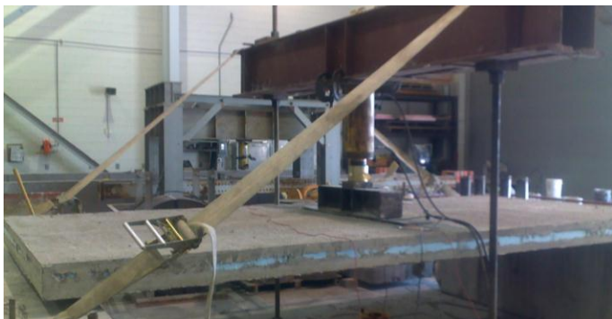
Figure 8: Testing and failure mode of panel A
