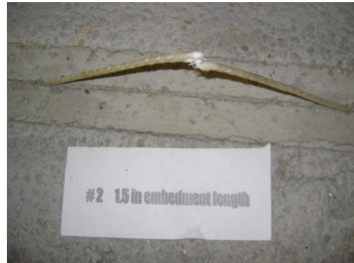
Figure 15: Rupture of the tie
