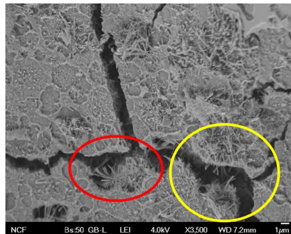
Fig.12 SEM Image for Group 3 Sample (Showing MWNT pull-out and MWNT being too short to span over the micro defects)
