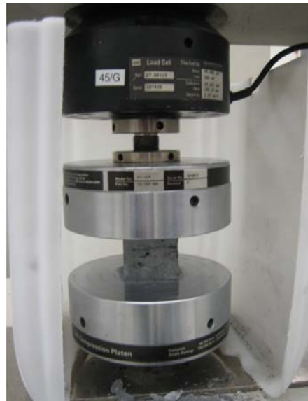
Fig. 3 Cube Compression Test on 45/G Test Machine
