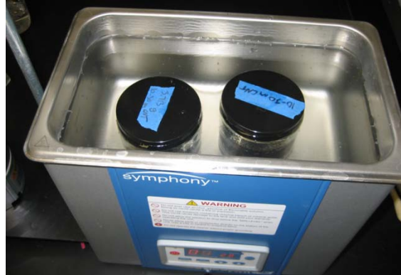
Fig. 2 MWNT Dispersion Using Ultrasonic Bath
