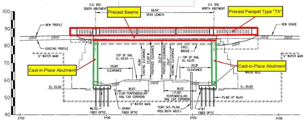
Fig. 5. Bridge Elevation.
