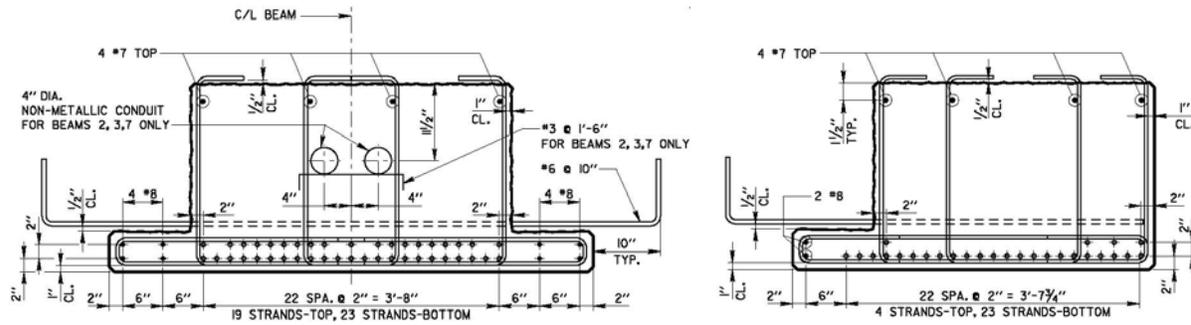
Fig. 11. (a) Interior Beam Section.
