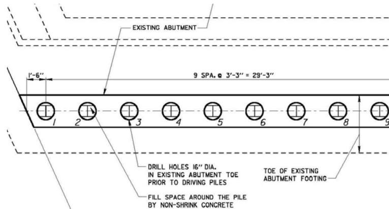
Fig. 7. Abutment Piling Plan.
