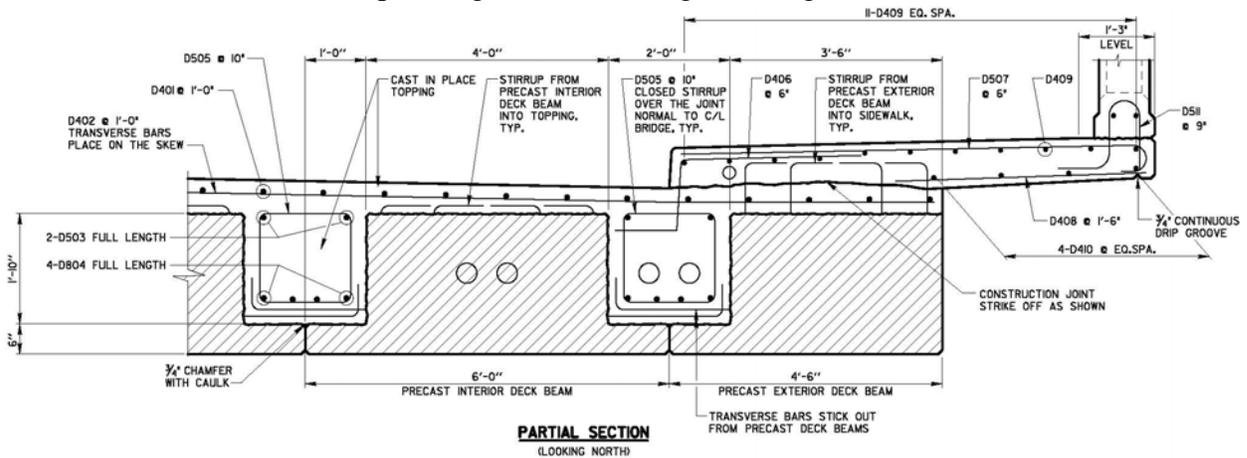
Fig. 10. Superstructure Partial Section.
