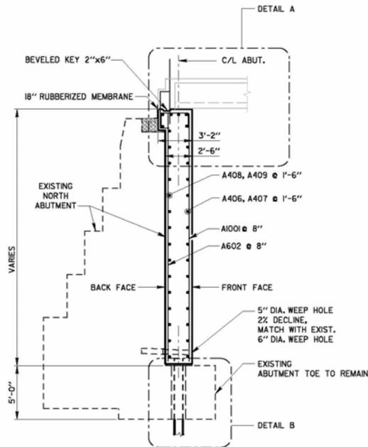
Fig. 6. Typical Abutment Section.
