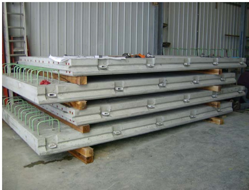
Fig. 7 Precast Deck Panels (at fabricator's plant)
