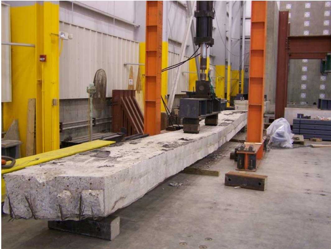
Fig. 13: Destructive Test of Beam 16
