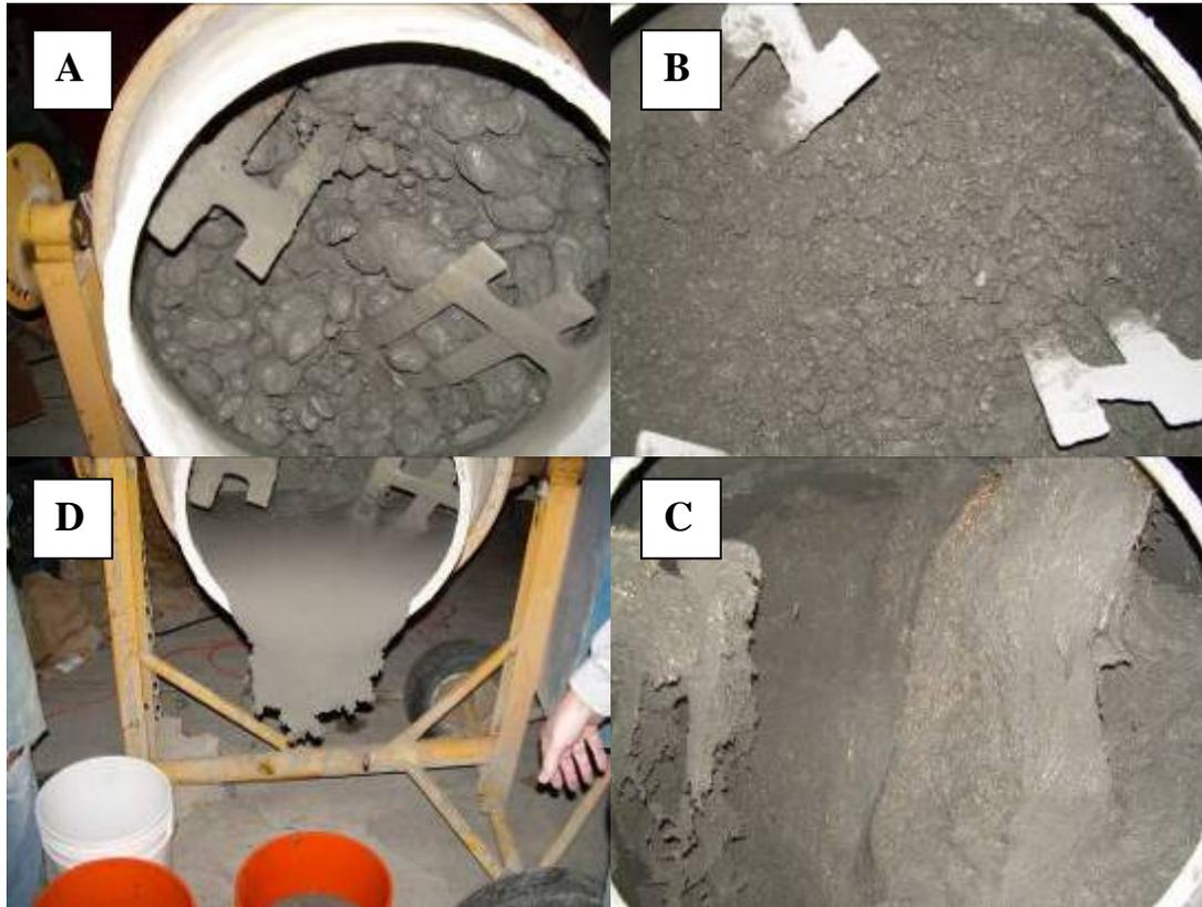
Fig. 2 Batching Ductal® in a Rotating Drum Mixer.
