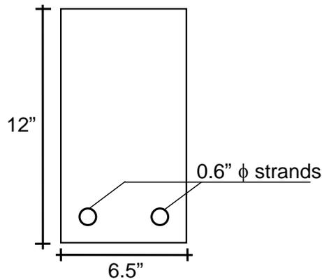
Fig. 1 Typical Beam Cross Section
