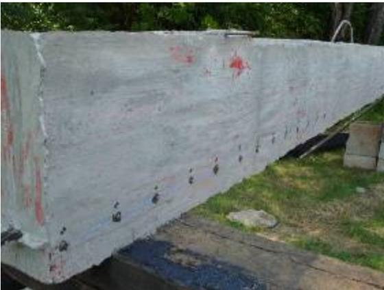
Fig. 3 DEMEC Target Locations
