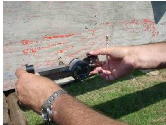
Fig. 4 DEMEC Gauge Reading
