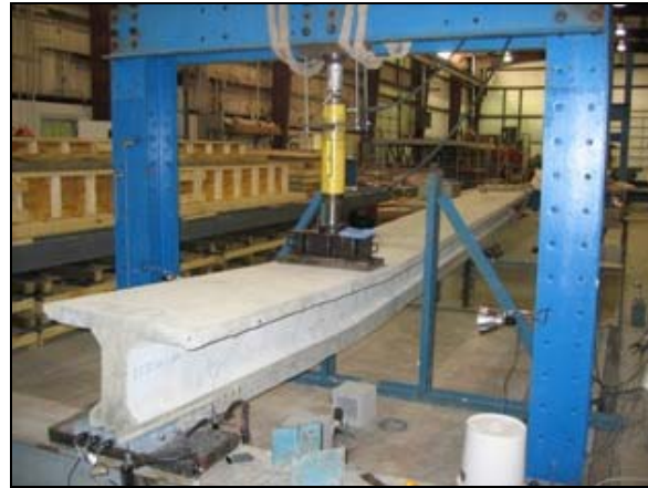
Fig. 12 Single Point Bending Test Setup
