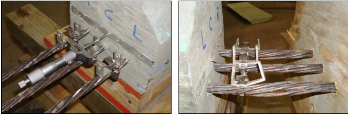
(a) (b) Fig. 11 End Slip Measurements Setup
