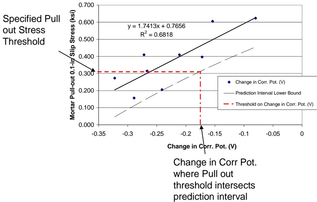
Figure 1 - Threshold determination using the prediction interval for Change in Corrosion Potential (Confidence Level = 90%).
