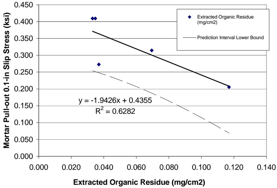
Figure 5 - Prediction Interval for Organic Residue when FTIR analysis indicates organic residue is primarily stearate (Confidence Level = 90%). Threshold not possible.
