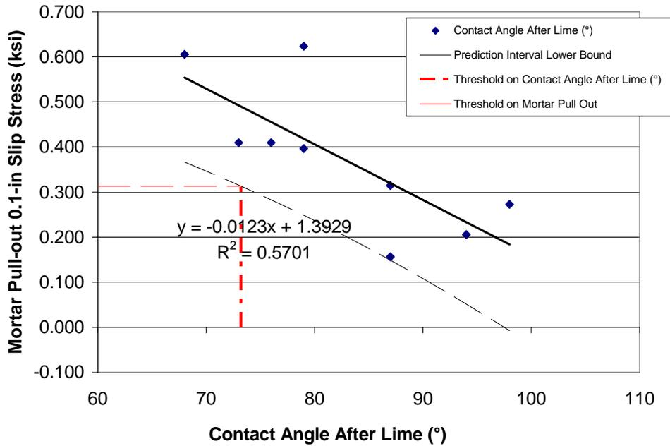
Figure 3 - Prediction Interval for Contact Angle After Lime Dip (Confidence Level = 90%).
