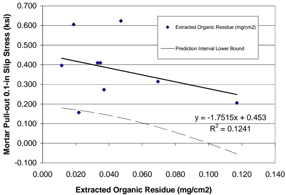
Figure 4 - Prediction Interval for Organic Residue (Confidence Level = 90%). Threshold not possible.
