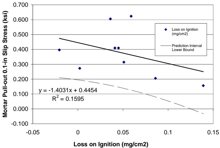
Figure 2 - Prediction Interval for Loss on Ignition (Confidence Level = 90%). Threshold not possible.
