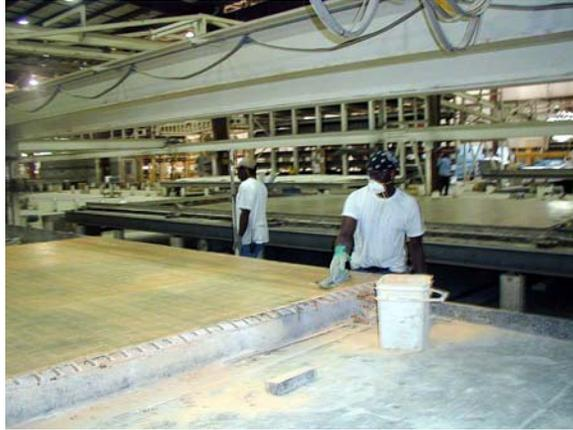
Fig. 13. Edges are floated and tooled by hand
