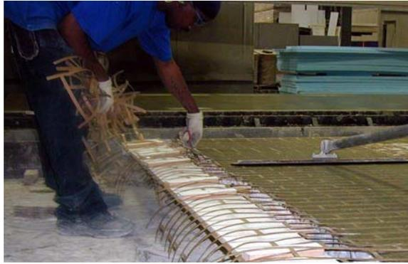
Fig. 8. Stencils are cut to fit along edges
