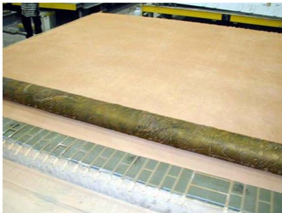
Fig. 14. A long roller applies texture across the entire panel width
