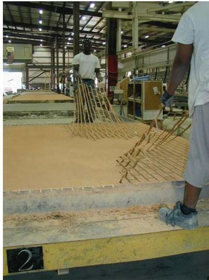
Fig. 16. Stencils being removed, exposing the pattern
