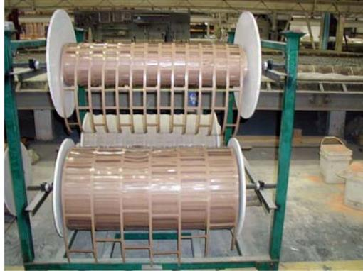
Fig. 1. Stencils are available in large rolls to facilitate mass production of precast concrete
