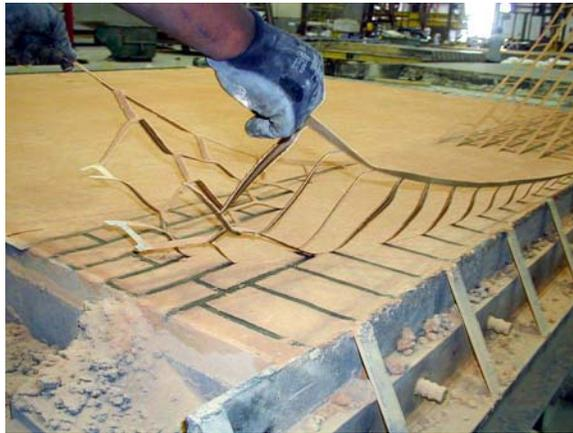
Fig. 15. Checking stencil release before removal
