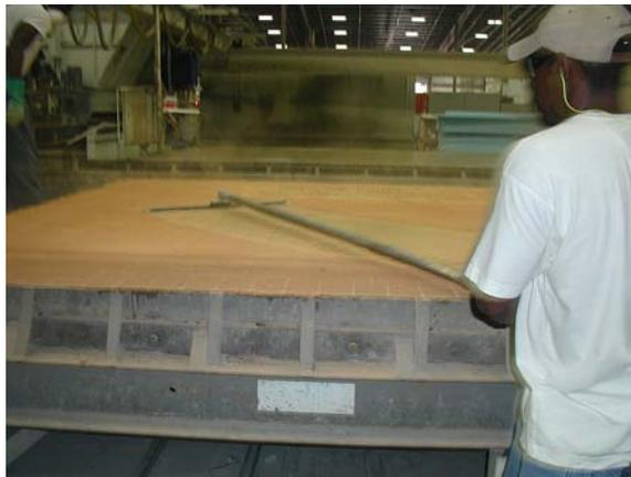
Fig. 12. Color hardener is floated over stencils
