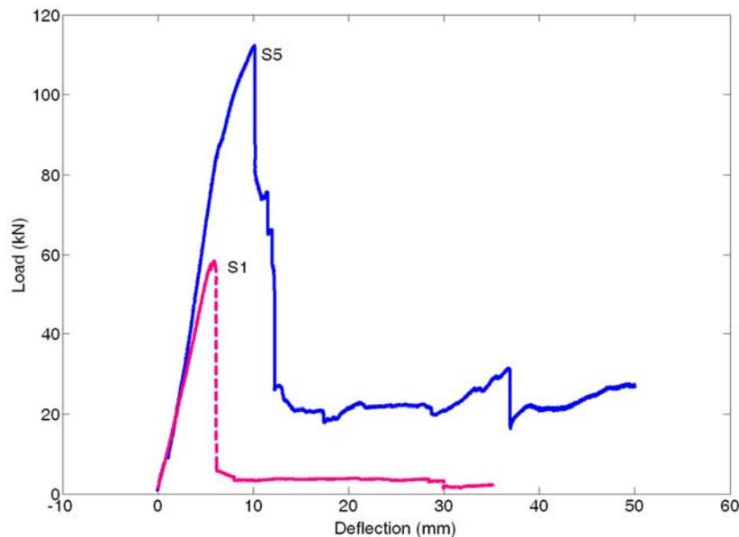
**Fig. 3 Load-deflection curves for control beam S1 and CFRP strengthened beam S5**
