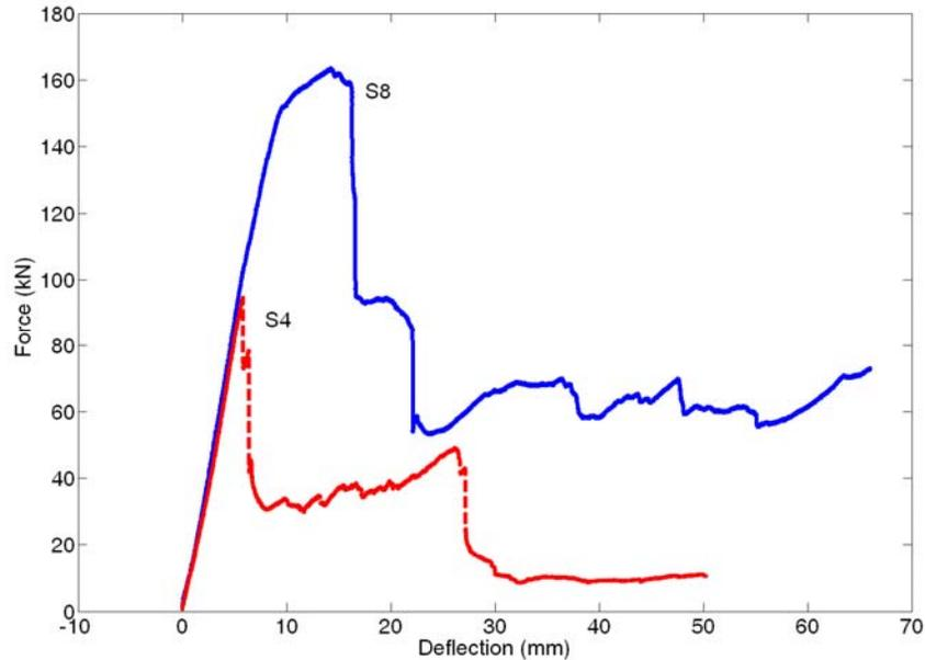
**Fig. 6 Load-deflection curves for control beam S4 and CFRP strengthened beam S8**
