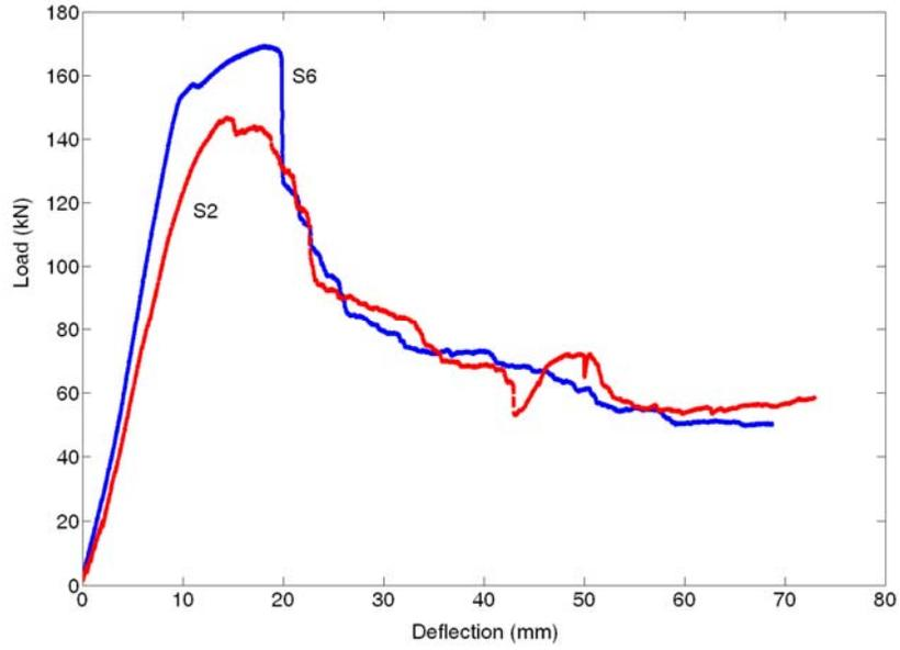
**Fig. 4** Load-deflection curves for control beam S2 and CFRP strengthened beam S6
