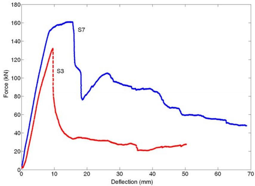
**Fig. 5** Load-deflection curves for control beam S3 and CFRP strengthened beam S7
