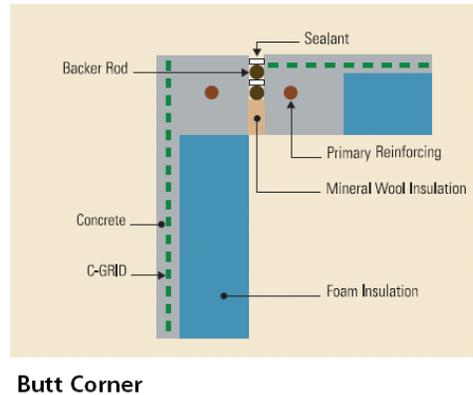
Fig 3 Double caulking at joints for moisture control
