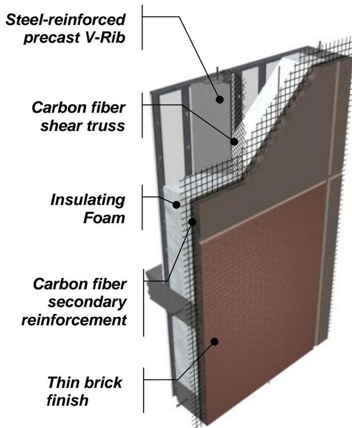
Fig. 1 Lightweight cladding reinforced with carbon fiber
