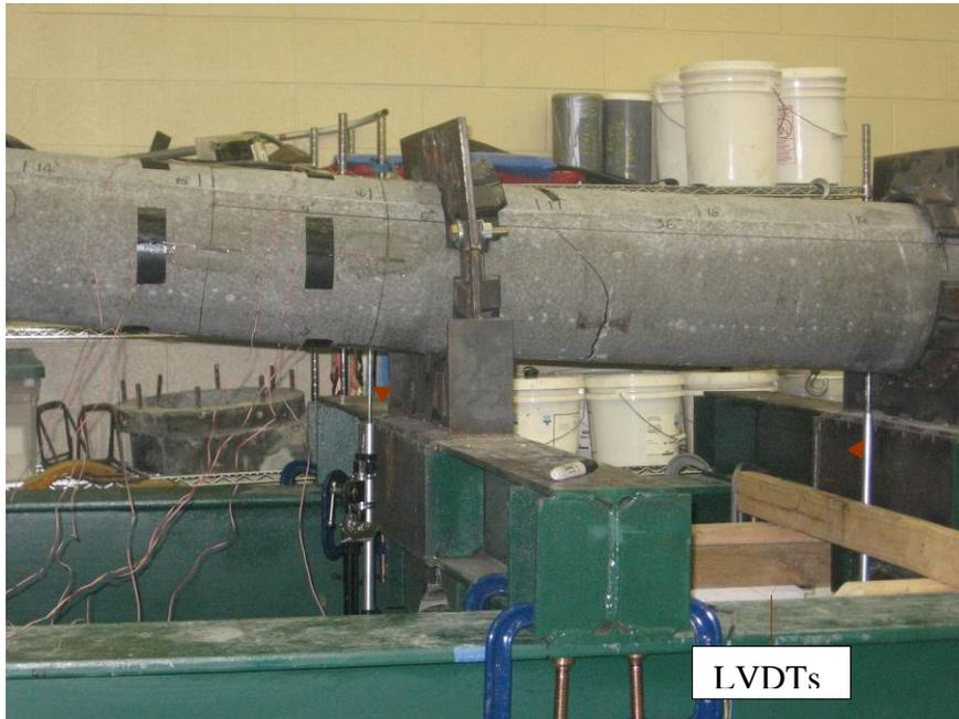
Figure 13: LVDTs for deflection measurements and corrections
