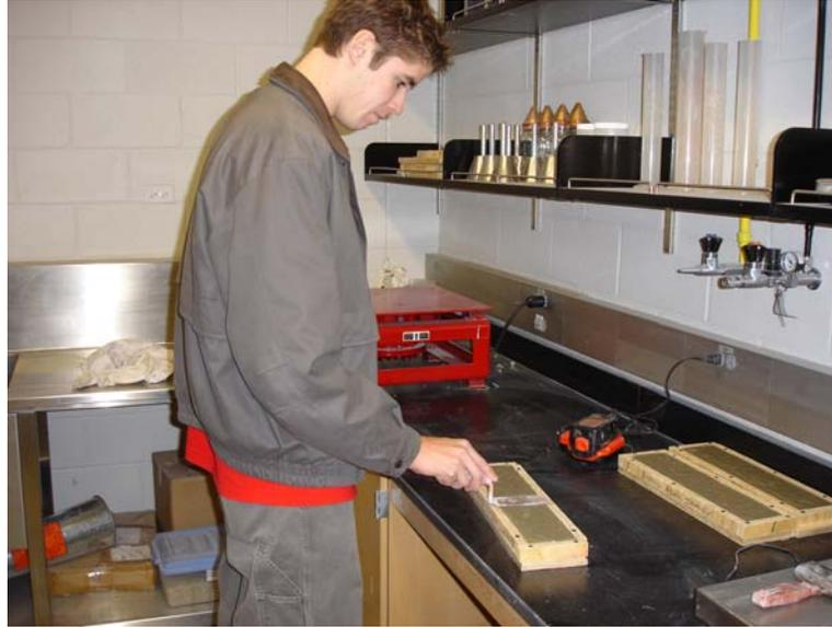
Fig. 4 Casting ECC Bar Specimens
