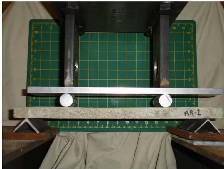
Fig. 5 Four Point Bend Test
