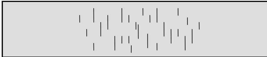
(b) Nonlocalized Cracking of ECC Bars
