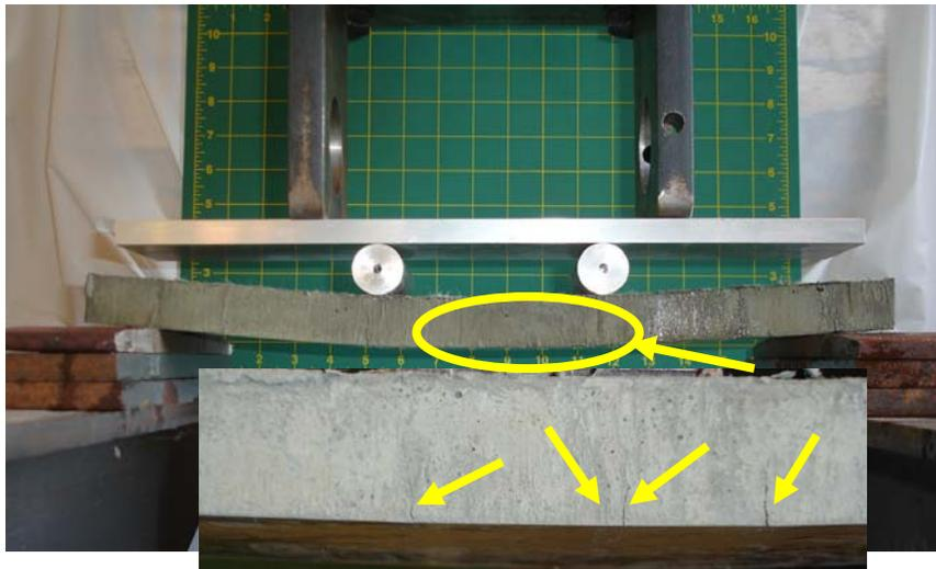
Fig. 7 Flexural Cracking of PVA Bar
