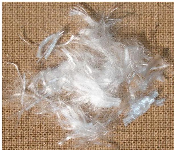
Fig. 2 Micro-fibers (Fibermesh 150 shown)
