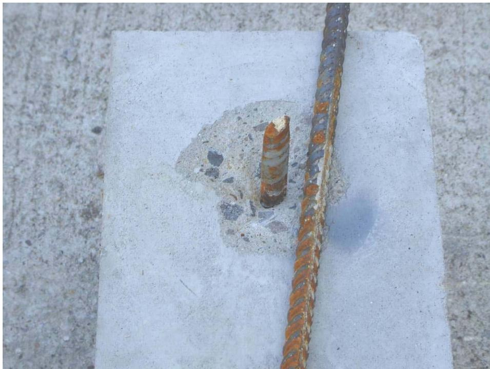
Figure 9: Steel Failure
