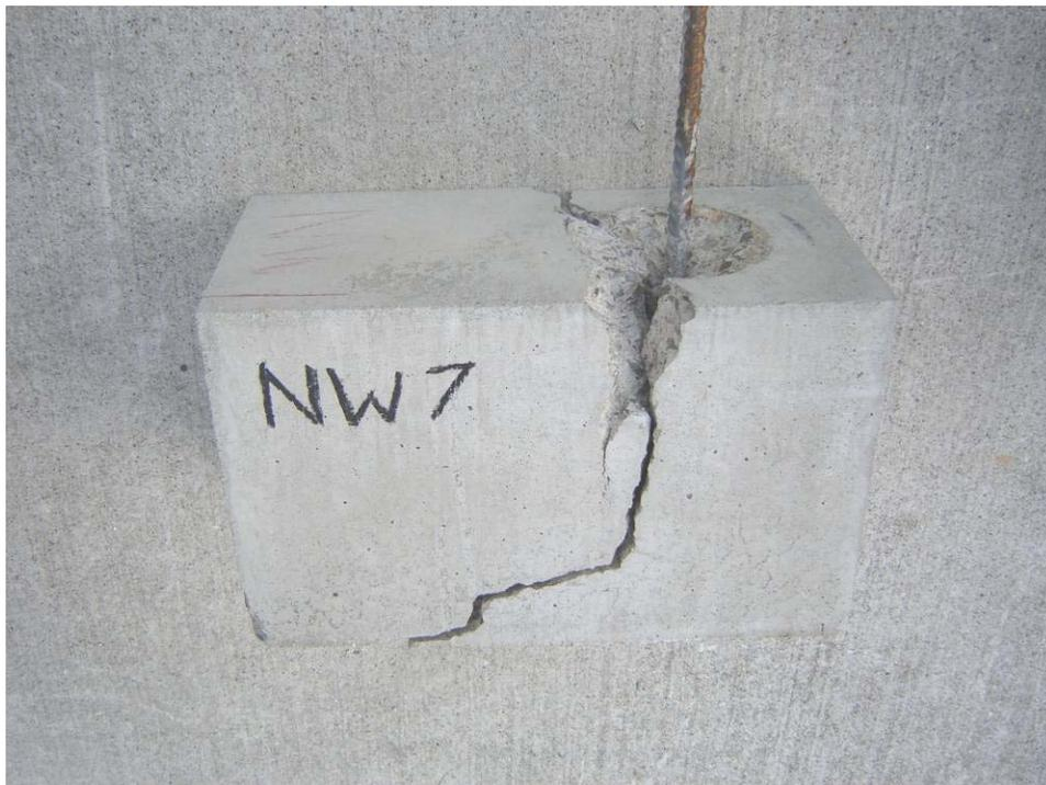
Figure 7: Concrete/Bond Failure
