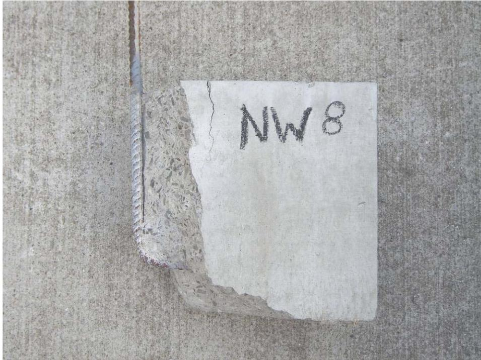
Figure 8: Concrete Bond Failure
