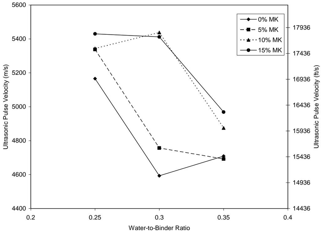
Fig. 5 Effect of Water-to-Binder Ratio on Ultrasonic Pulse Velocity in Concrete.
