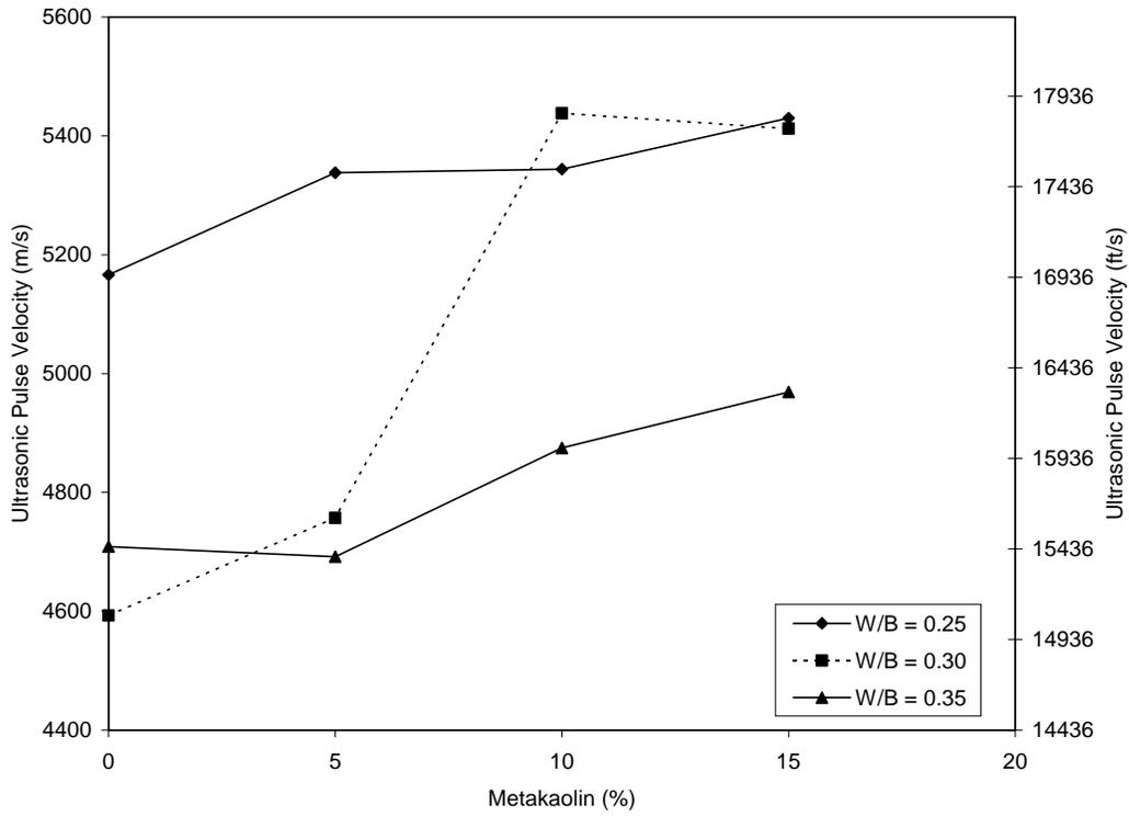
Fig. 4 Effect of Metakaolin Content on Ultrasonic Pulse Velocity in Concrete.
