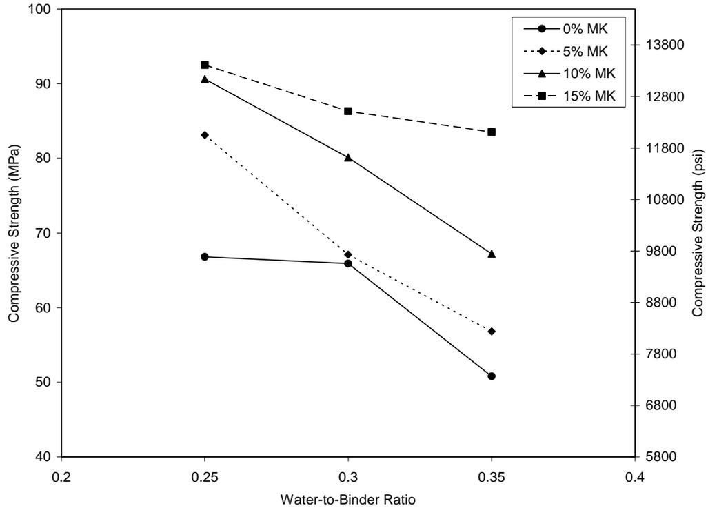
Fig. 3 Effect of Water-to-Binder Ratio on Compressive Strength of Concrete.
