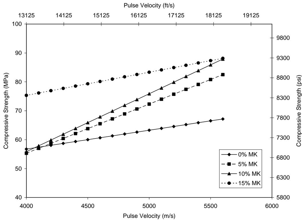
Fig. 6 Graphical Representation of Pulse Velocity and Compressive Strength Model for various Metakaolin Contents.
