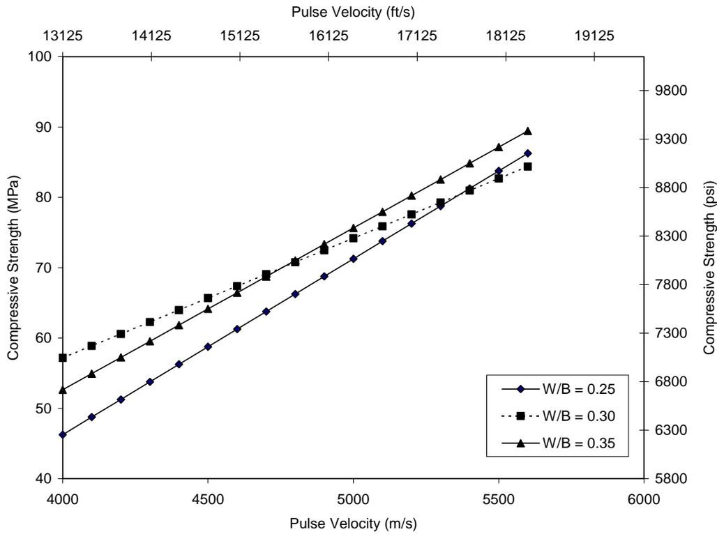
Fig. 7 Graphical Representation of Pulse Velocity and Compressive Strength Model for various Water-to-Binder Ratios.
