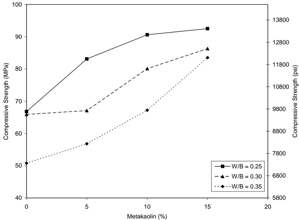
Fig. 2 Effect of Metakaolin Content on Compressive Strength of Concrete.
