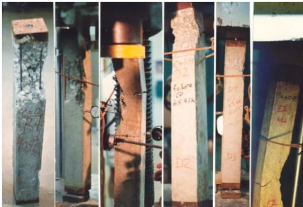
Figure 12 Some of the columns after testing curves
