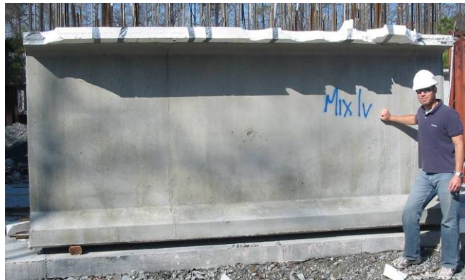
Figure 2. 13-ft. BT-72 mock-up
