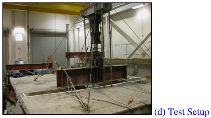
Fig. 12. Fabrication, Installation & Test Setup of the Full-Scale Bridge
