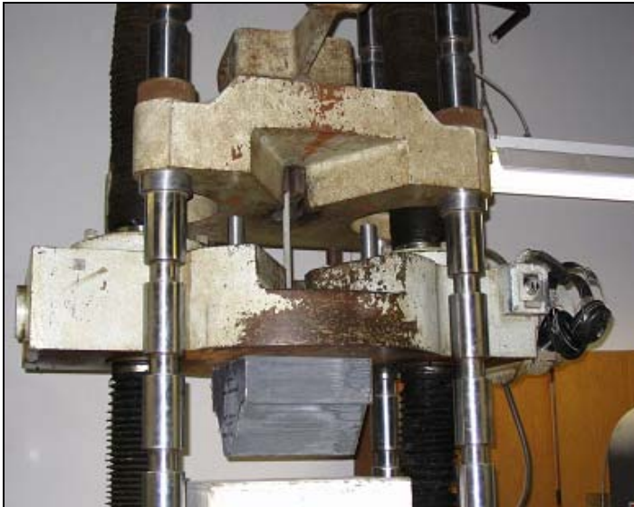
Fig. 6 Test set-up for pullout capacity of GFRP in UHPC block
