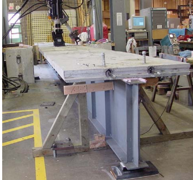
Figure 7: Test configuration for the composite beam test.
