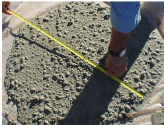
Fig. 4 S.C.C.’s “spread” is measured
