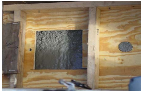
Fig. 8 Self-filling under horizontal bulkhead
