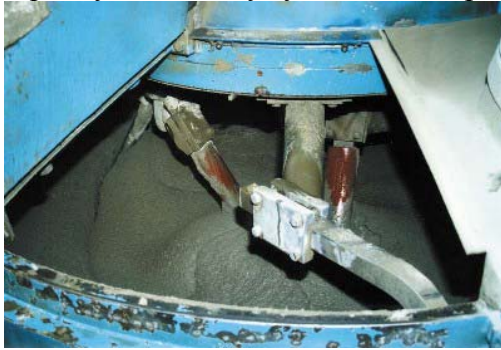
Photo 8 – Mixing in progress
