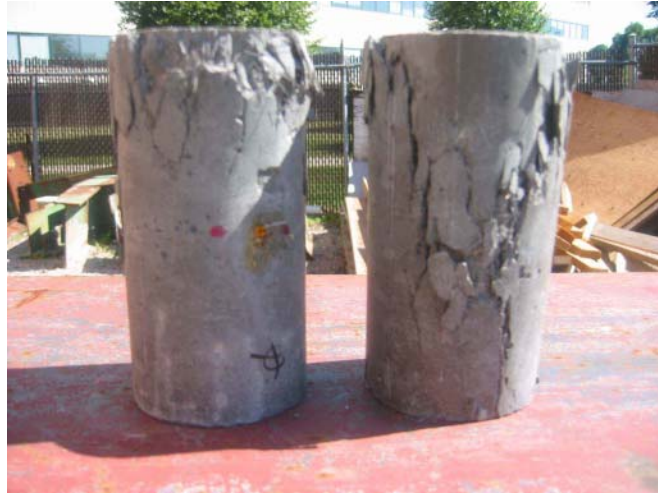
(b) Samples after failure
