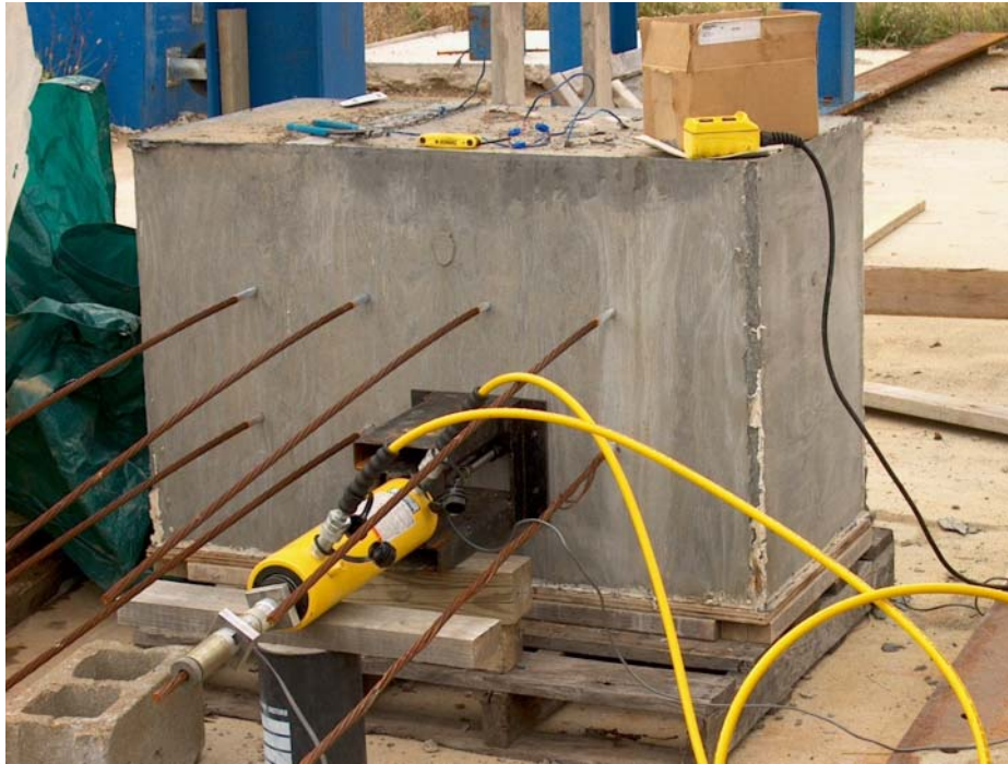
Fig. 2 - Pull-out Test Sample
