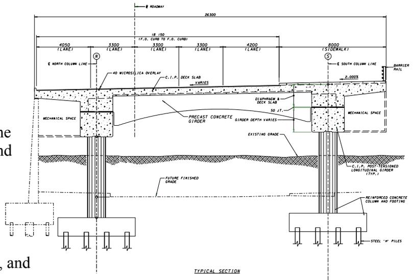
Fig. 5 – Cross section of Second Street Bridge.
