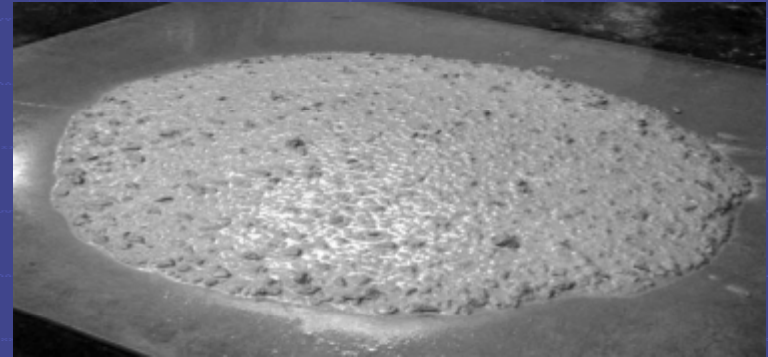
VSI = 1 – Concrete shows slight bleeding, observed as a sheen on the surface
