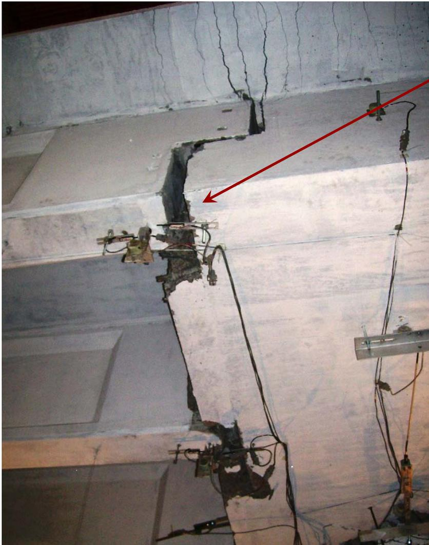
Opening up of as-built connection under positive-moment loading
