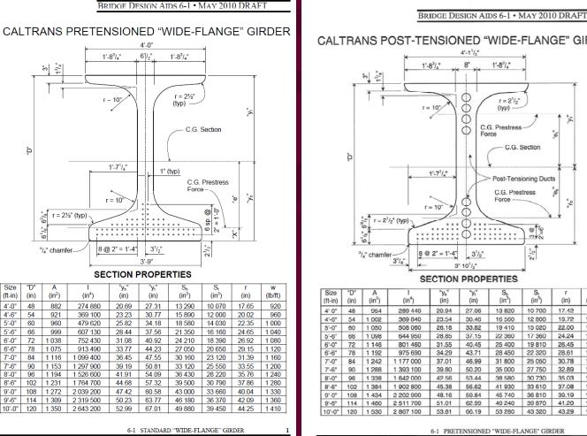
CALTRANS POST-TENSIONED "WIDE-FLANGE" GIRDER 4'-11/2" 1'-83/4" 8"  $r = 2^{1}/2^{n}$ Ó (typ) C.G. Prestress Φ Force C.G. Section Post-Tensioning Ducts C.G. Prestress Force œ CT N @ 2" = 1'-4" 31/2" 3'-101/2" SECTION PROPERTIES
