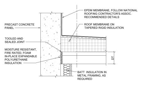
PRECAST CONCRETE WITH BATT INSULATION NTS
