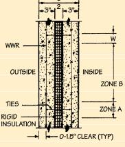
Fig. 15 Metal tie thermal bridges
