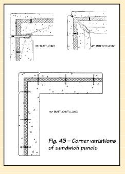
the concrete panels. Anything connected or adjacent to the sandwich panels must be able to accommodate such movement. If it is essential that they are in the same theoretical plane, it is suggested that they be framed around with material which is not flush with the walls, similar to suggestions for corner columns. A door or window frame can be attached to the inside wythe since the movement is confined to the exterior wythe.
