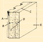
The above design example shows how to calculate R-value and U-factor for a wall using material R-values taken from Tables 2 through 7.
