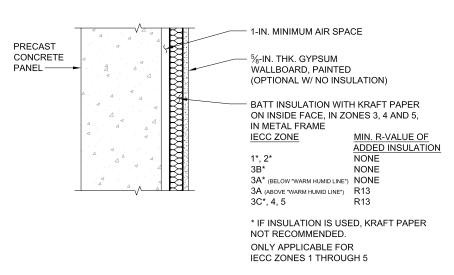
PRECAST CONCRETE WITH BATT INSULATION NTS
