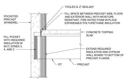
PRECAST CONCRETE WITH BATT INSULATION
