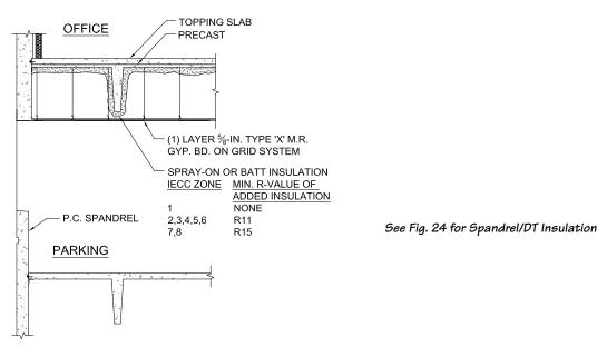
C PRECAST CONCRETE WITH BATT INSULATION
