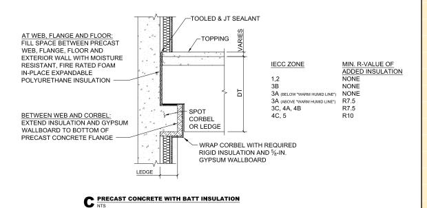
Fig. 28 – Typical Loadbearing Spandrel with Corbel/Dapped DT Detail
