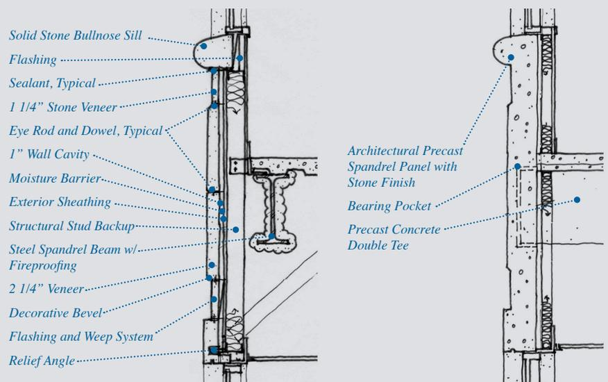
and water infiltration, mold, connection corrosion, weep accommodation, etc.) given the number and coordination of different building trades required. Complicated exteriors like the veneer wall involve more individual parts and materials, resulting in more intensive maintenance requirements over the life of the building.
