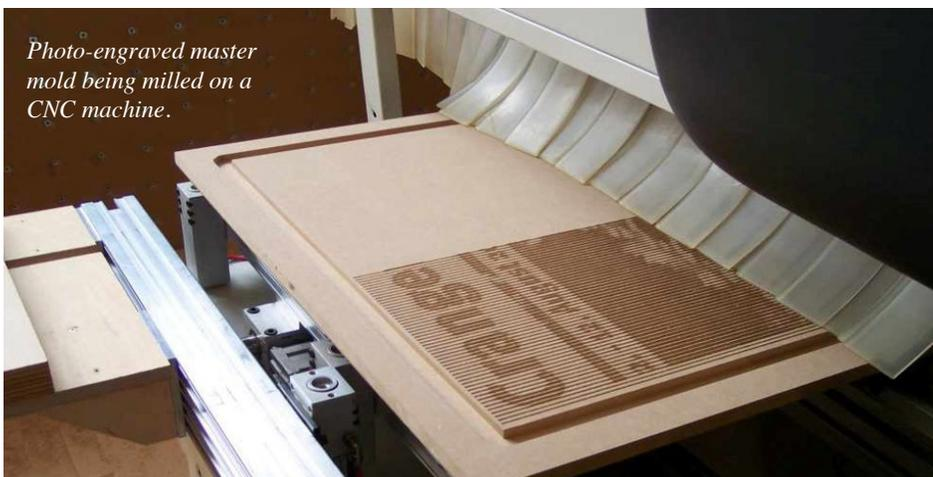
*Photo-engraved master mold being milled on a CNC machine.*
