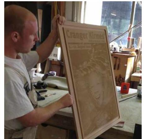
*In the offset light, the image on the photo-engraved master mold can be seen. A formliner will be made from this and then cast in concrete.*
