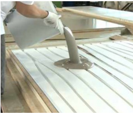
This image shows the precast concrete panel that was made from the custom rope formliner.
