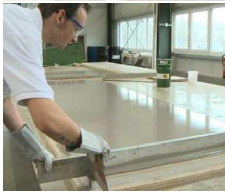
Next, the formliners are screeded to provide a smooth level back.
