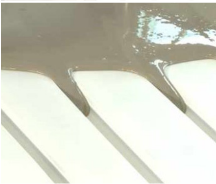
These two images show polyurethane formliners being made. Liquid polyurethane is poured onto the master mold.
