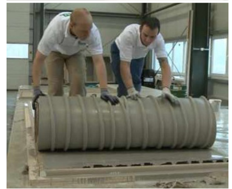
After 24 hours, the formliners can be demolded and rolled onto a tube for transportation to the QA/QC area for final inspection prior to shipping to the customer.
