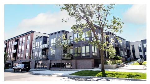
Taracon Precast manufactured over 60,500 SF of hollowcore, 130 inverted tee beams, and 56 columns for the foundational support, elevator shafts, and multi-level flooring. Designers were able to use precast stepped ledge beams and columns with varying haunch heights for balcony and amenity decks. Precast concrete was selected for this project because of its durability and load-bearing capabilities.
