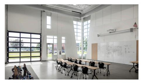
Overhead garage doors facilitate the movement of large equipment and enable the expansion of hands-on learning activities. Each door also integrates a secondary storm panel, ensuring a bright, open learning environment under normal conditions while providing essential protection during severe weather.
