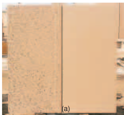
Fig. 5. Use of 4 ft (1.22 m) samples to establish acceptable range of color and texture. Concrete made with 3/8 in. (9.53 mm) aggregate with retarded (left side) and acid etched (right side) finishes.
