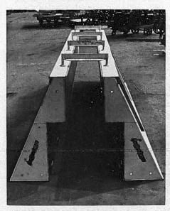
Food Machinery & Chemical Corporation of Lakeland, Florida, has introduced a new "Inverted T" steel casting form. The forms are supplied in 10-ft. lengths which can be connected to provide members of any required length. They are lock-up forms with pilot liners available for various bottom slab thicknesses. The forms produce a prestressed concrete unit designed for use with double tee roof and floor slabs.
