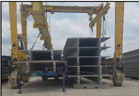
Typical loading arrangements for Double Tee product.
