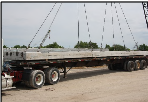
Typical loading arrangements for wall panel and hollow core floor product.
