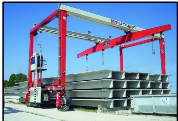
Typical stacking arrangements for double-tee product in storage yard
